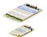
The 2-port M5e is designed for adding UHF RFID read/write capabilities to a wide range of products and solutions, from high-speed label printing and inlay testing, to stationary, mobile, and handheld computers. The M5e will transmit up to +30 dBm.
